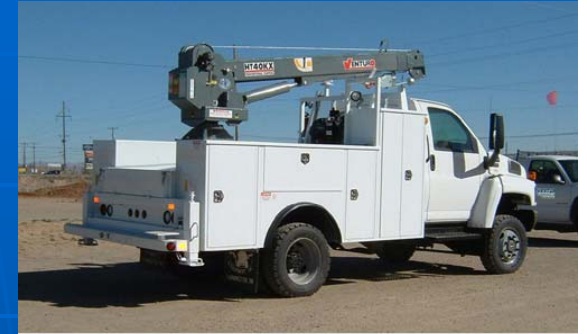
HT40KX-P Crane, HT40-133-TFC Crane Body, and 25000-CD Outrigger GM 5500 Chassis
